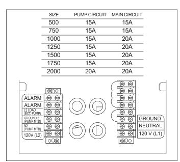
**NOTE:** This pump control is equipped with a delay on break typically set for 3 minutes, but can be adjusted between 0.1 and 10 minutes.
